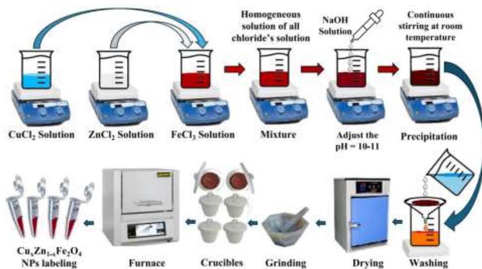
Figure 1. \text{Cu}_x\text{Zn}_{1-x}\text{Fe}_2\text{O}_4 Nanoparticles synthesis process [11].
