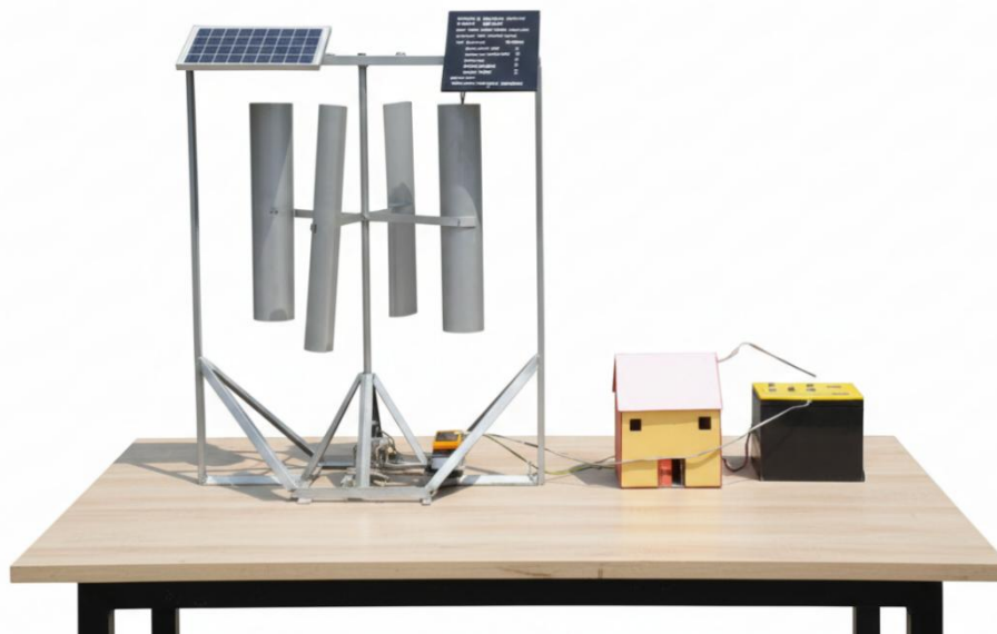
Figure 10. Fabricated Prototype of the Hybrid Solar-Wind Energy System showing Complete Assembly
